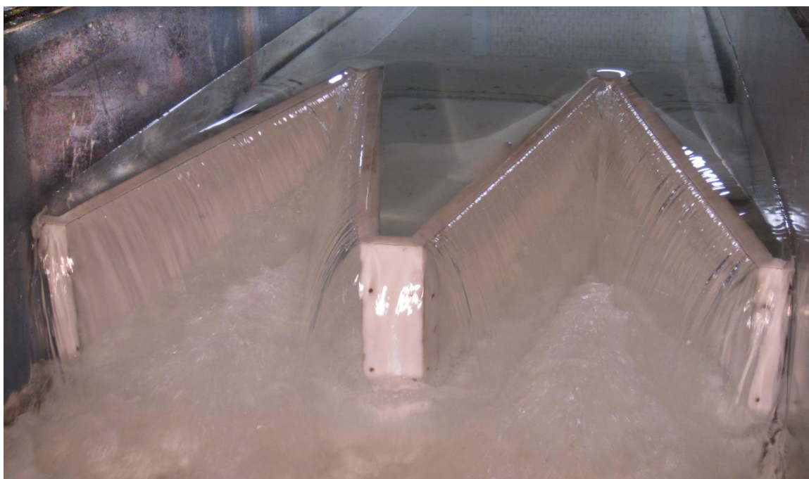
Fig. A-12. \alpha = 12^\circ , QR , A=1t_w , inverted orientation, H_T/P = 0.1 , photograph
