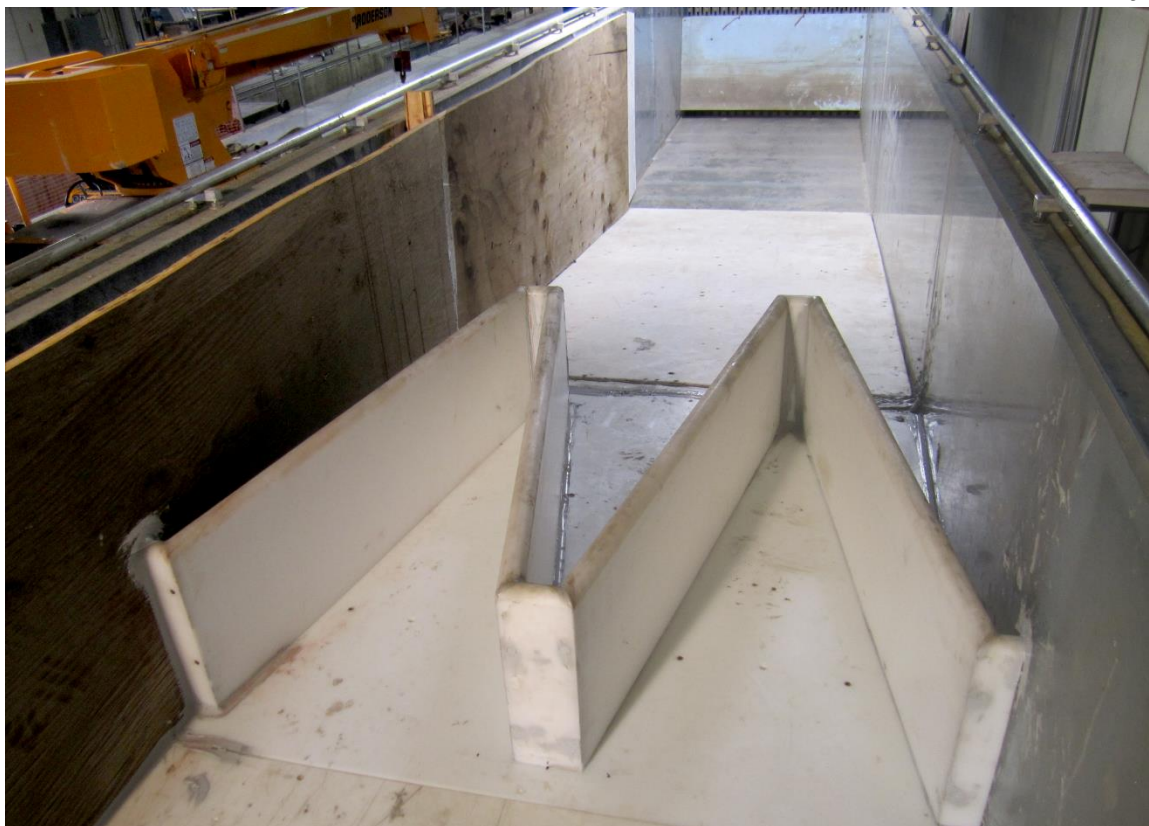
Fig. A-7. \alpha = 12^\circ , HR , A=1t_w , inverted orientation, false wall, photograph
