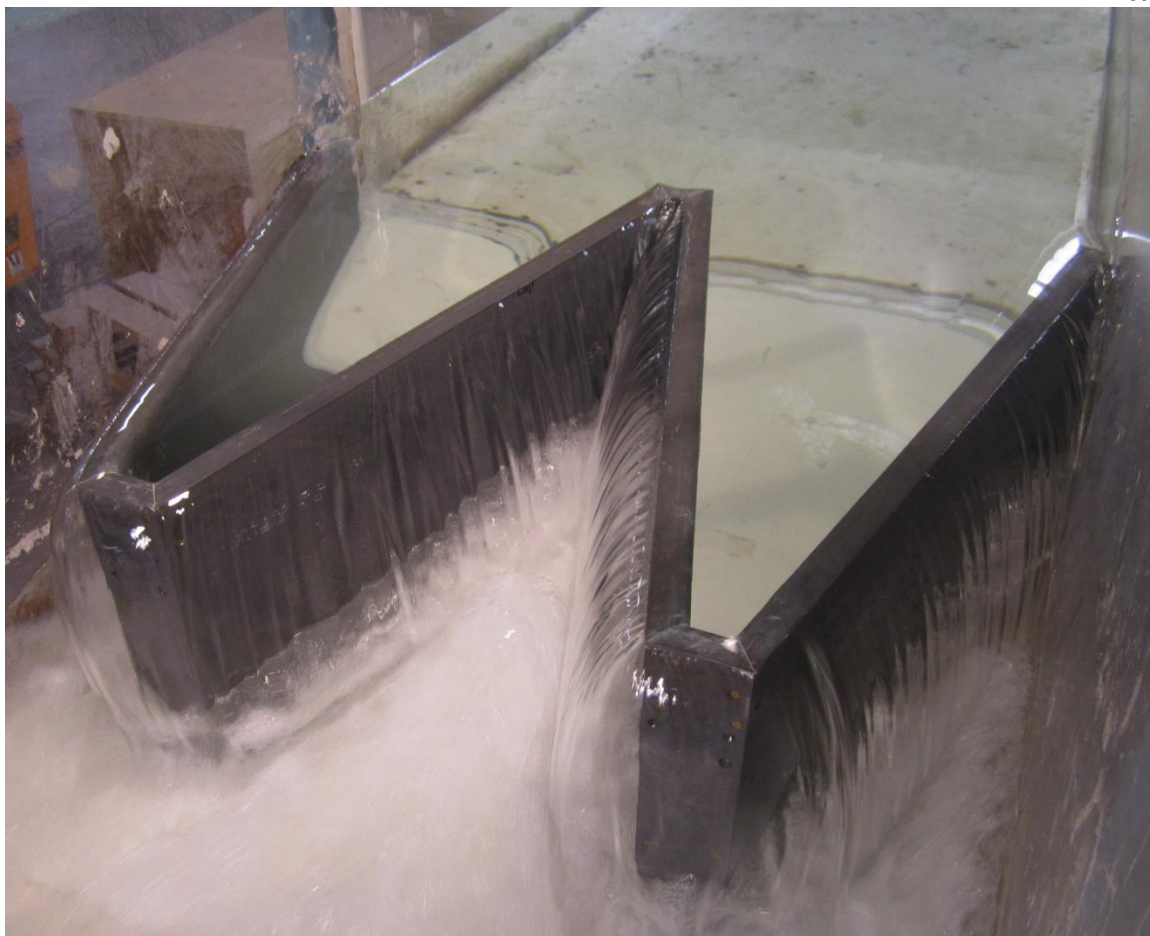
Fig. A-21. \alpha = 15^\circ , QR , A=1t_w , normal orientation, H_T/P = 0.1 , P=15 in, photograph
