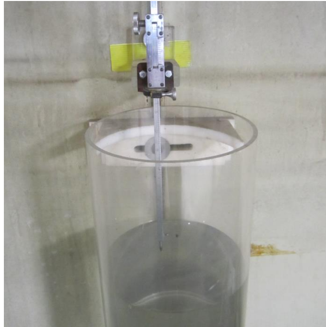
Fig. 11. Stilling basin with point gage
